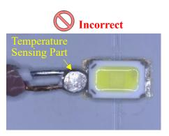
The wires are thick. The temperature sensing part is too large.
